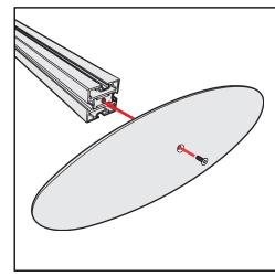
Base Plate & Extrusion Connection
