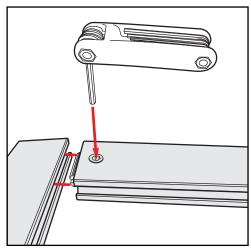
**Extrusion & Lock Connection**
